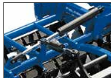
Hydraulic depth adjustment from the cab using the master / slave cylinders (optional).
