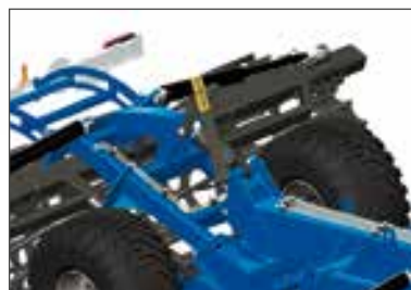
Hydraulic adjustment of working depth with optical indicator.
